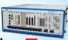
**40-923A** 19-Slot PXI Modular Chassis
