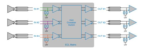
The KSD0490 is capable of switching data rates up to at least 650 Mbit.
